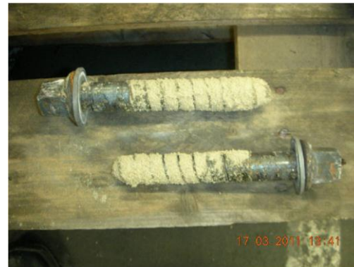
Greased screws covered with sand
